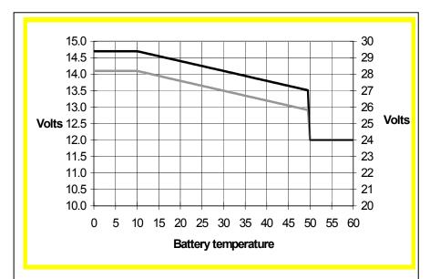
Default output voltages for Float and Absorption are at 20°C. Reduced Float voltage follows Float voltage and Raised Absorption voltage follows Absorption voltage. In adjust mode temperature compensation does not apply.
