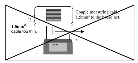
The correct connection of the measuring cables is very important. If they are incorrectly connected, the battery guard will activate too early and the WhisperAir will switch itself off.
