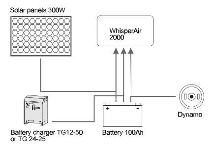
While sailing on the engine it is possible to simply charge and maintain the battery using the dynamo. The capacity of the dynamo should be a minimum of 60A. However, the solar unit will provide at least 300 Watts or a 50A for 12 Volt or 25A for 24 Volt battery charger may be used to recharge the battery, should you wish to remain stationary for a longer period.
