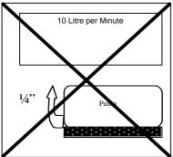
The water pump must have a capacity of at least 20 litres per minute and be fitted with a hose of 34". The number of litres passing through the air-conditioning unit must be at least 10 litres per minute. Moreover, (sea)water with a temperature of maximum 35°C is required. The AirWhisper will not be able to lose the extra heat and will turn itself off if the (sea)water is warmer than this temperature.
