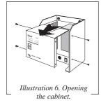
To adjust the charge voltage unscrew the four countersunk screws in the sides of the Pallas, with a Phillips screwdriver, and pull the panel outward.
