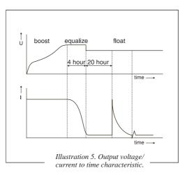
hours the batteries will have been charged to 100% of their maximum capacity. After the "equalize" period is over, the "equalize" LED will be turned off, the "float" LED will light up and the "float" period will start.
