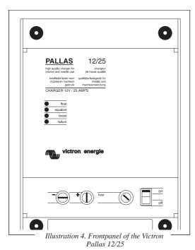
Automatic charging will commence approximately 10 seconds after the mains have been connected and the switch "charger on" is set in the "on" position; the LED "on" will light up immediately.
