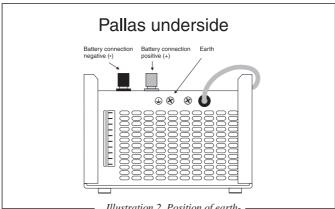
Illustration 2. Position of earthing screw on the Pallas 12/25
