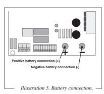
and thicker. The combined resistance of the two cables must not exceed 4 milliohms.
