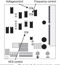
voltage may be adjusted by turning potentiometer P2 (top right) to the left ("-") or to the right ("+"). For the accurate measurement of the output voltage you will need a true - RMS multimeter or a moving iron voltmeter.
