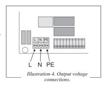
The inverter will be damaged if another alternating current (e.g. from a generator) is connected to the 230V output.
