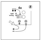
Ensure that all switching between different 230 V<sub>AC</sub> power supplies (e.g. shore generator) takes place by means of DOUBLE-POLE switches. Otherwise the Atlas may be damaged.
