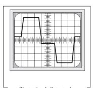
Illustration 1. Outputvoltage waveform during "on" mode.
