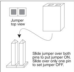
Illustration 10. Placing the jumper.
