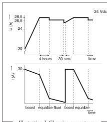
Illustration 3. Charging current waveform in relation to battery voltage.
