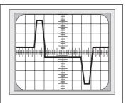
Illustration 2. Output voltage waveform during "AES" mode.
